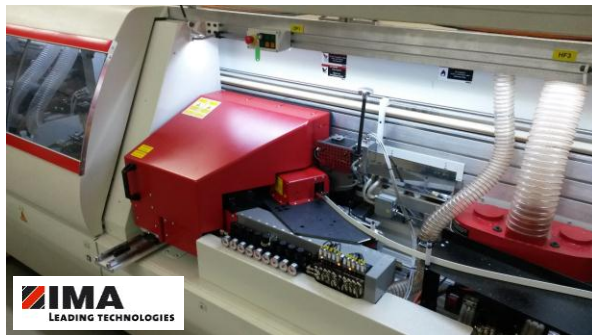
Figure 18 IMALUX direct laser system on through-feed machine from IMA Klessmann GmbH for small and medium-size workshops
