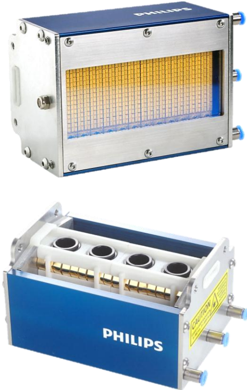
Figure 4 A 4.8 kW VCSEL module containing 12 emitters with 24 individually addressable zones
